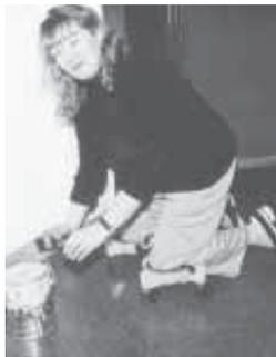
**Rolling spring-loaded kneepads make it easy to scoot around without crawling or standing up.**
