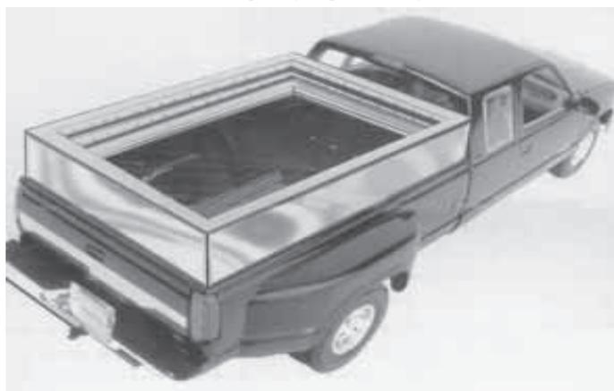
**Unit consists of four 12-in. high aluminum panels that bolt to top of bed rails. "Lets you haul bigger, bulkier loads than you can with a cargo cap or tarp," says John Chechuck.**
