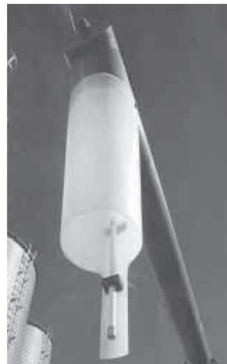
**Wireless bin sensor bolts on in place of auger's original down spout. When grain contacts a sensor, a transmitter automatically triggers an alarm on tractor.**
