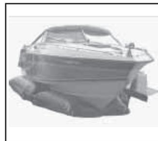
**Air-Dock uses air-filled bladders to lift boat. It can be inflated using either DC current from boat's battery or regular 120-volt AC.**
