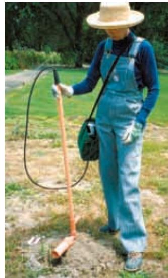
Oxygas uses an 8-lb. cordless air compressor to force gas from a CO<sub>2</sub> cartridge or vehicle exhaust down into underground tunnels.
