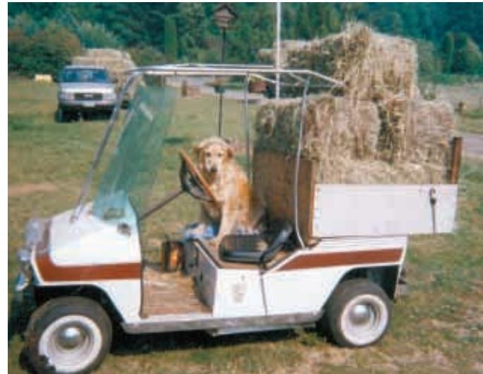
Joe Taylor added a wood dump box on back of this electric-powered golf cart for hauling lawn clippings, bales, etc.
