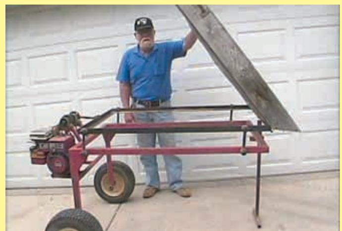
Motorized screening cart is small enough to fit in a pickup, allowing Snyder to take it on-site rather than having to bring material home to be separated.
