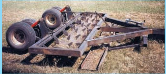
Aerator has a 20-in. dia. drum with 8-in. steel tines welded onto it. I-beam in front of drum drags down mole hills and small piles of manure.
