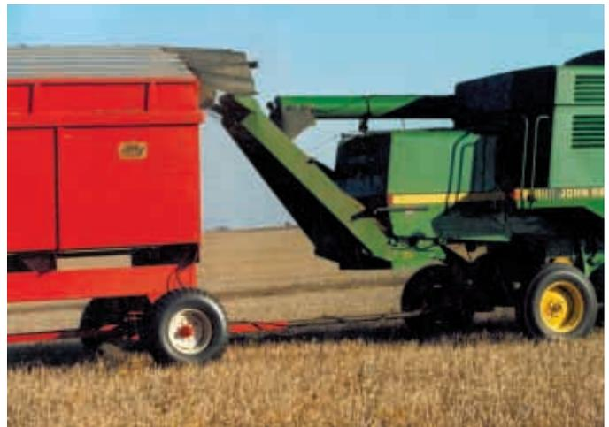
Straw goes through chopper on back of combine and up a chute into a side-dump silage wagon. Chaff is still collected with Redekop unit.
