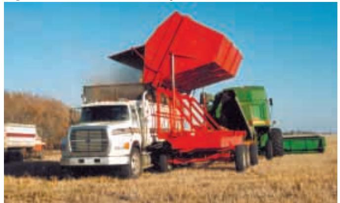
Side-dump silage wagon delivers material into truck.
