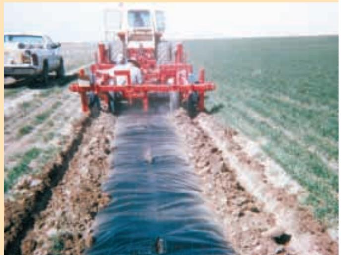
Heavy-duty machine plants trees into sod, lays down a plastic subsurface drip irrigation line, and puts a black plastic weed barrier over the top, all in one pass.
