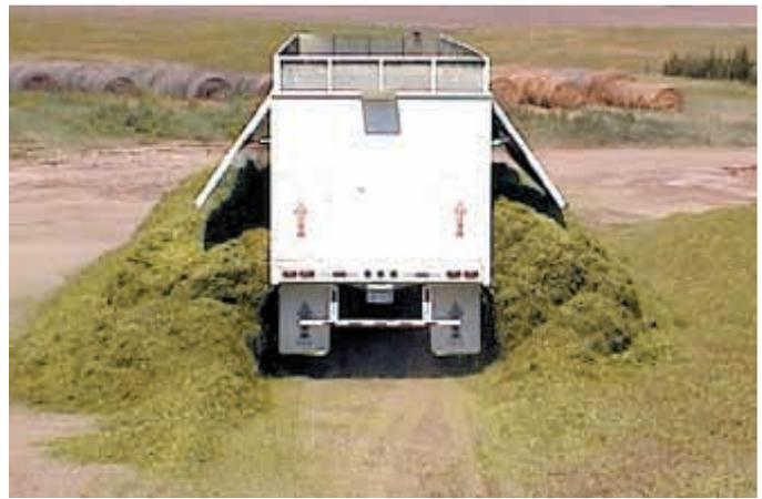
Design lets you unload on-the-go on uneven terrain because the load slides evenly down the "V" floor and out both sides of trailer.
