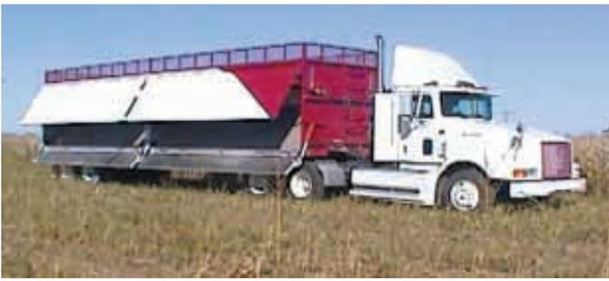
Trailer has an inverted "V" floor that's angled at 50 degrees and two independent sets of side doors. Upper door is hinged at top and opens hydraulically.
