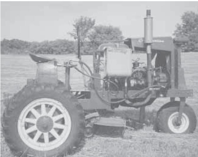
Loren Smith's 1930's tractor is a reminder of the days when it was as common to build a tractor as it was to buy one. It has a Model A Ford engine and 3-speed transmission with an IH 2-speed truck axle. "This gives it six speeds forward and two reverse," he says.
