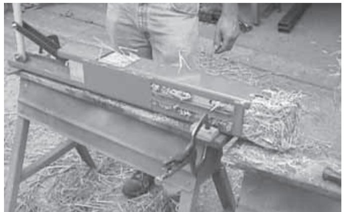
Mini "hand feed" replica baler produces bales that measure just 8 1/2 by 4 1/2 by 3 5/8 in. and weigh about 2 lbs.
