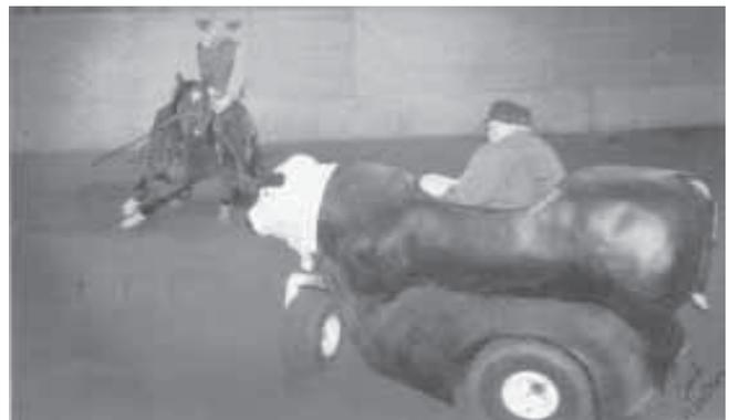
Mechanical bull has a fiberglass body that looks like a steer. Rider uses a pair of levers to control speed and steering.
