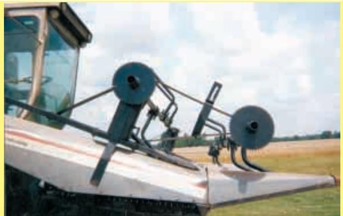
First reel grabs loose stalks and pushes them onto gathering chains. Reel behind it helps move stalks into cross auger.
