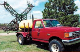
"I saved thousands of dollars over the cost of a commercial sprayer," says Leon Sowers, who built his own pickup sprayer. It's equipped with a 60-ft. long "X-fold" boom.
