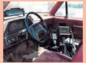
Boom nozzles are regulated by a Tee Jet 844 controller that mounts in the cab.
