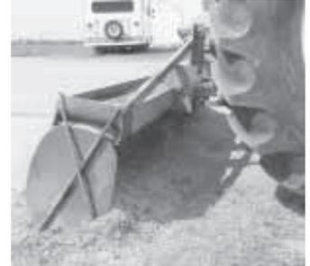
**He used a 10-in. I-beam as the main frame and added a 3-pt. hitch and 3/16-in. thick plate steel for the sides. The blade is from a highway department snowplow.**
