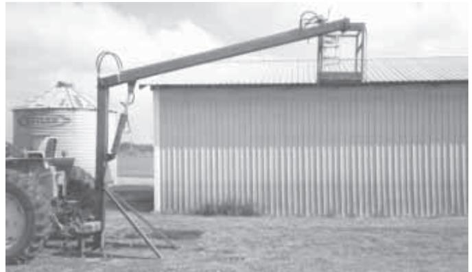
**Shop-built, hydraulic-operated man-lift is attached to an old 3-pt. bale mover. Steel bucket mounts at end of 12-ft. boom.**
