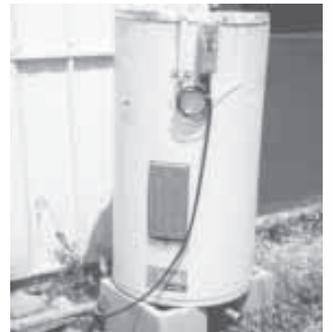
Electric scalding was made by modifying an old 50-gal. hot water heater
