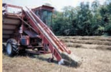
Arledge built bale hauler on the frame of an IH combine. Bale cage slopes to the back for easy unloading. When rear gate is opened, bales fall out all at once.
