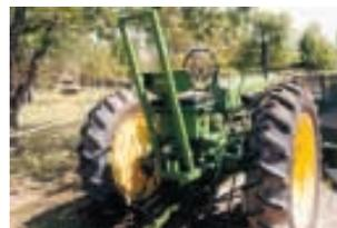
Steanson used square tubing and steel plate to build a rollbar on his Deere 2-cyl. tractor. "The narrow rollbar doesn't interfere with getting on and off the tractor," he says.
