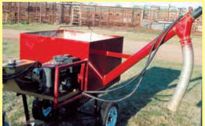
Leon Sowers uses this ATV-pulled wagon to feed calves after they're weaned. Unloading auger is powered by hydraulic power unit that's driven by an 8 hp gas engine.
