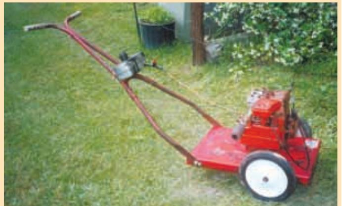
Engine mounts on the frame of an old pressure washer. Insecticide is stored in a small plastic tank mounted on rig's handles.
