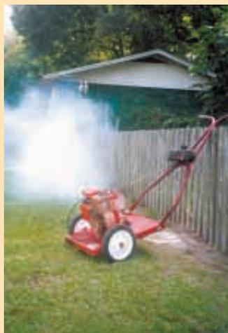
Fogger uses heat from a small gas engine to vaporize oil-based insecticides. Engine exhaust then blows the fogged insecticide out the side.
