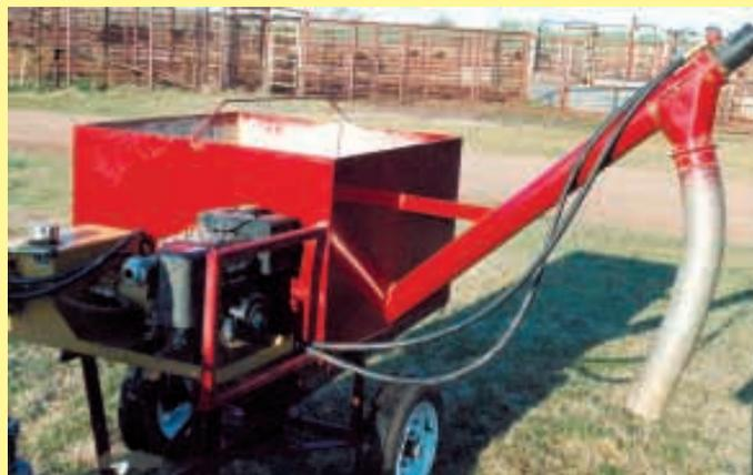
Leon Sowers uses this ATV-pulled wagon to feed calves after they're weaned. Unloading auger is powered by hydraulic power unit that's driven by an 8 hp gas engine.
