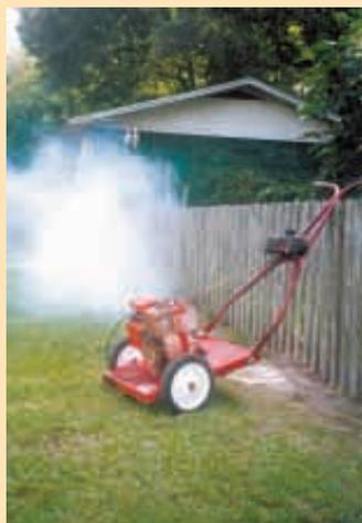
Fogger uses heat from a small gas engine to vaporize oil-based insecticides. Engine exhaust then blows the fogged insecticide out the side.
