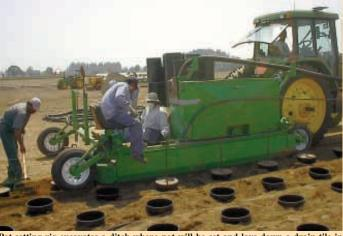
Pot-setting rig excavates a ditch where pot will be set and lays down a drain tile in bottom of ditch. Irrigation pipes are run alongside.
