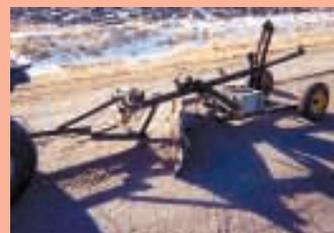
Blade angle is adjusted by changing the position of a pin. An electric winch mounts ahead of blade.
