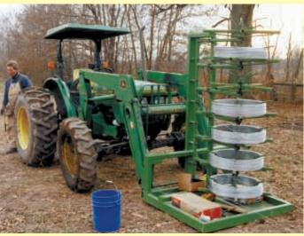
Custom-built fence machine quick-taches to Halbrook's front-end loader and holds up to seven spools of wire. Operator drives backward to unroll wires off spools.
