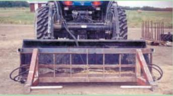
Triangular-shaped arms, fitted with bale spears, mount to the frame on heavy hinges. A pair of hydraulic cylinders move arms in or out.
