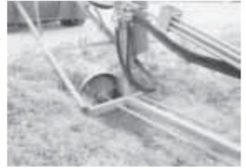
An orbit motor rotates the brush as it slides into culvert. Six 6-ft. extensions can be added to brush for a total reach of 40 ft.
