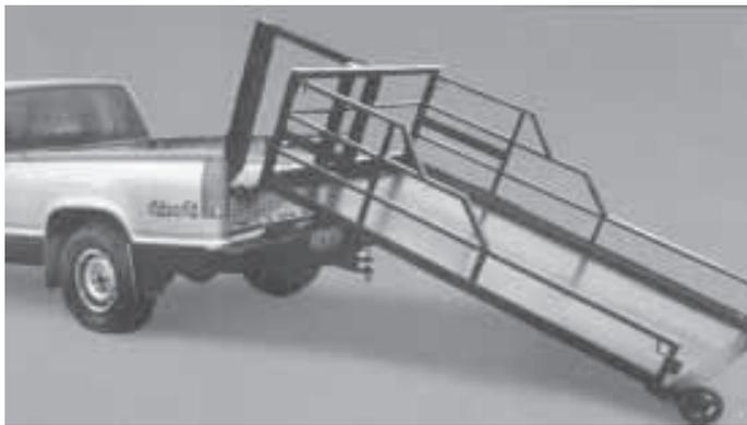
“Super Deck” platform rotates back at a 45 degree angle until wheels on back of platform contact the ground.
