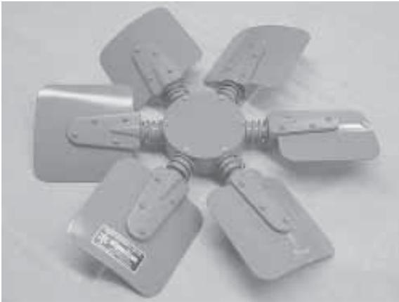
Reversible fan is used to blow out radiators when operating in dusty and trashy conditions.
