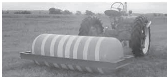
**Ed Grafke used a 500-gal. propane tank to make this roller, which he uses to level the turf on his airplane runway.**
