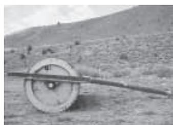
**Design keeps the weight down and also makes roller easier to pull because most of the weight is on the outer edge.**
