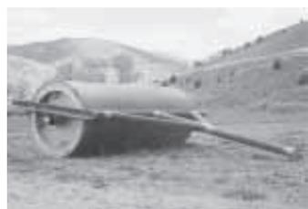
**Randy Pentz put a 3-ft. dia. piece of pipe inside a 4-ft. dia. pipe and filled the 6-in. gap between them with concrete.**
