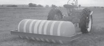
Ed Grafke used a 500-gal. propane tank to make this roller, which he uses to level the turf on his airplane runway.
