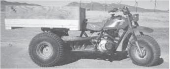
Jeff Hoard extended the frame on his 3-wheel ATV and mounted a dump bed on it.
