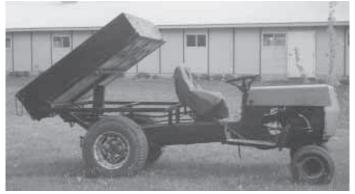
Lennie Buscho converted an old Montgomery Wards 10 hp garden tractor into a handy chore vehicle equipped with a hydraulic-operated dump box.
