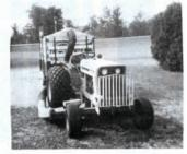
Kohler gas engine. The blower works like a hammermill and consists of a shaft fitted with 4 metal blades that are about 4 in. wide at the shaft and taper out to about 12 in. wide. The engine direct-drives the blower shaft. I attached a boot to the mower deck that connects up to 8-in. dia. flexible tubing. Grass and leaves are pulled up through the blower blades and then blown up into the wagon.
