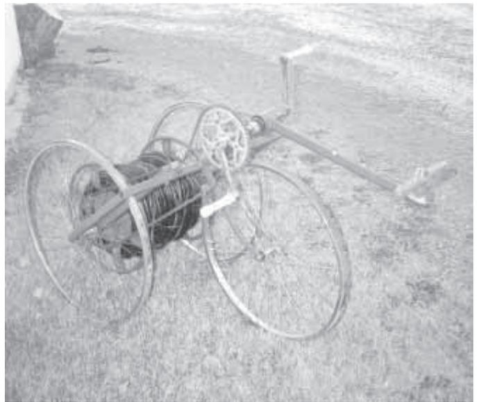
Graydon Dennis built this “tricycle” cord reel out of old bicycle parts and a commercial cord reel. By holding onto a handle with one hand and turning a crank with the other, he’s able to let out cord as he walks along.
