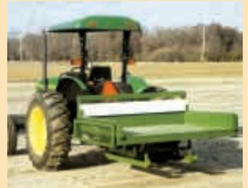
Unit mounts on steel skids. Sideboards can be folded up, down, or pointing straight out to the sides.
