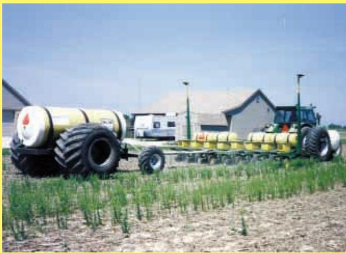
Liquid fertilizer cart was built from the frame of an old C2 Gleaner combine. Big flotation tires on the rear axle minimize compaction.
