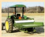
Unit mounts on steel skids. Sideboards can be folded up, down, or pointing straight out to the sides.
