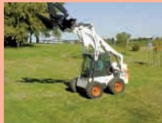
Blade on the "Timberline" tree shear can be rotated, allowing you to trim tree branches up to 15 ft. off the ground.
