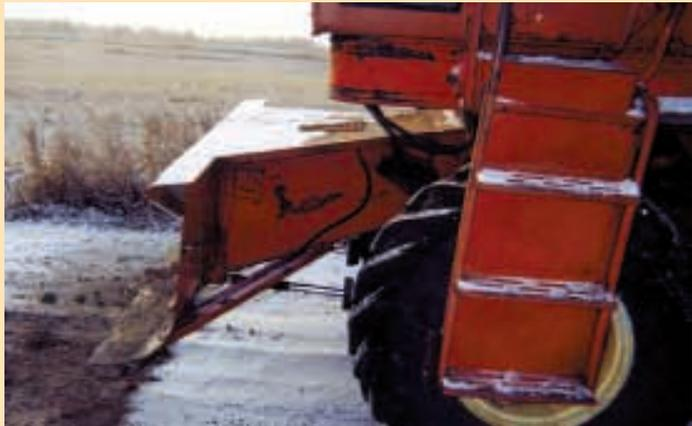
Sickle bar bracing plates were cut up to make a solid curved plow blade.
