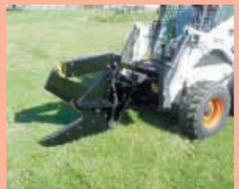
To rotate shear, operator pulls a spring-loaded pin and manually rotates the balanced frame. Pin automatically snaps into hole when alignment is correct.
