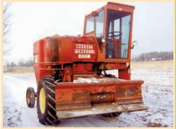
To convert a Massey 300 combine to a snowplow, Adophson cut off the ends and part of the platform, cutting it back to the shape of a plow blade.
