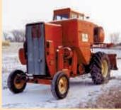
He removed the grain sieves and rearpart of housing as well as the unloading auger, using sheet metal to close everything up.
