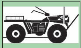
Flat steel bar runs from back of ATV to front, where it angles up at 45 degrees, extending about 30 in. in front of machine.
