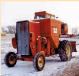
He removed the grain sieves and rear part of housing as well as the unloading auger, using sheet metal to close everything up.
