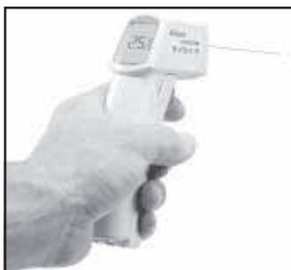
Unit instantly measures surface temperature of almost any object using a beam of infrared light.
