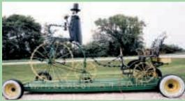
I came up with the idea to build a high wheel bicycle similar to the ones from the late 1800's. It's built entirely out of used barn cleaner chain links as well as rebar and flat iron. Everything is welded
