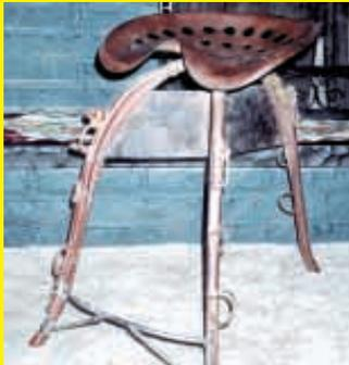
in. thick mild steel plate gussets, located about 3 in. under the seat. To stop the two front legs from spreading I used 3/8-in. dia. rod tack welded to the hames about 4 in. from the bottom. My neighbor is 6 ft. 6 in. and weighs 240 lbs., but the chairs don't even flex under his weight. They're extremely comfortable. (Wally Bunt, Rt. 7, Hwy. 61 4093, Thunder Bay, Ontario, Canada P7C 5V5 ph 807 475-9161)
