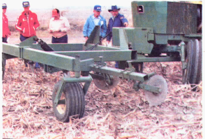
Nine coulters mount in front of the tractor to cut through trash before chiseling.
