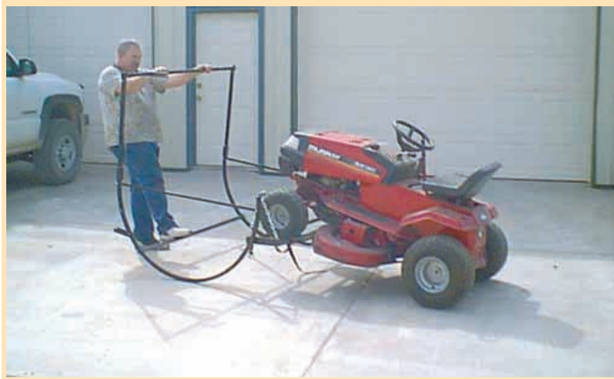
After hooking mower onto tray, you pull back and push down on cross bar until it touches the ground. A pair of safety stops lock bar in place.
