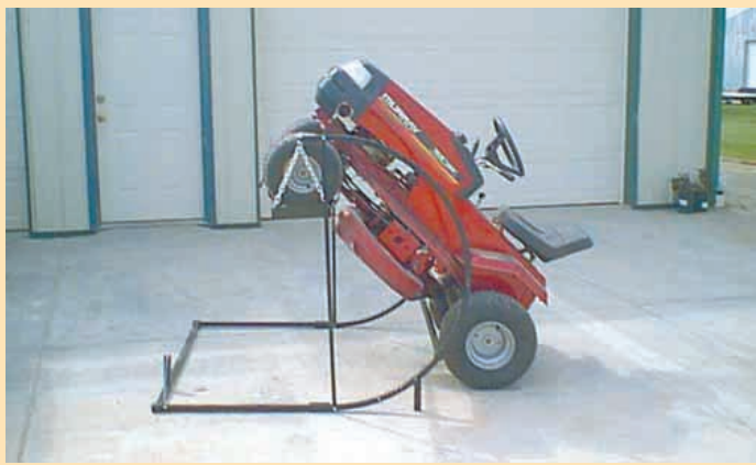
Once the Mower Lift is in place, you can clean the deck, sharpen the blades or do other maintenance work on the mower.
