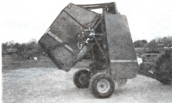
Kicker pushes the bale far enough backwards so you can close the rear door without backing up before you dump the bale.
