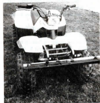
Folded tow bar is 34 in. wide, narrower than any 4-wheel ATV.
