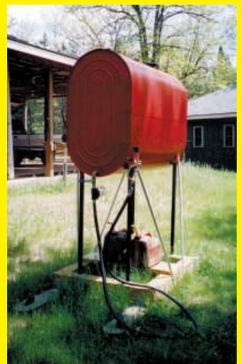
right on my own property. The tank is gravity fed and doesn't need a pump. It comes with a locking valve, fuel filter, 10-ft. hose, swivel nozzle, gauge and storage platform. The entire unit can be moved on a snowmobile trailer. I'm willing to build units for \$575. **(Dan Jacobson, 8913 Weaver Lake Dr., Pequot Lakes, Minn. 56472 ph 218 543-6623)**
