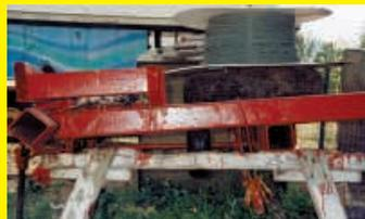
and a pto shaft. It works great with high tensile wire used for portable fencing and has saved us many hours of work.
