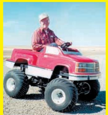
Several years ago I built these pedal-powered, fiberglass body monster trucks, which are designed to be driven by kids from 12 to 16 years old. All of them are chain-driven and have 2-speed transmissions. I built a total of 16 different pedal-powered monster trucks and also built pedal-powered, fiberglass body tractors for kids from ages 4 through 12.
