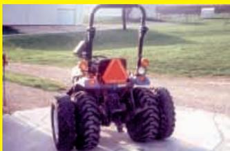
We had some stability issues with our small utility tractor when working on steep side slopes. We solved the problem by adding duals to the tractor. Now we can safely work on slopes with much less chance of tipping the tractor.
