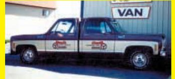
Here's a photo of a "two-way" pickup I put together in my shop. It's a 1978 Chevrolet 2-WD equipped with a 6-cyl. gas engine and a 4-speed manual transmission. I removed the bed and replaced it with an identical cab and nose, minus the engine. I also enclosed the area under the hood to make a big trunk.
