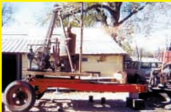
When I bought this "one horse" well rig made in the late 1800's, it was all wood. The tower and frame were wood and it had steel wheels. I installed a steel tower, an 8 hp engine, and mounted it all on a truck frame. It has 3, 12, 16 and 24-in. digging buckets. With reamers on the 24-in. bucket it will dig a 36-in. hole.
