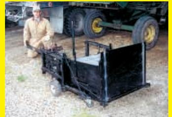
garden tractor or 4-wheeler to pull the 3-ft. wide machine. It consists of a rotating cylinder equipped with four paddle wheels and four rows of 2-in. long teeth. A 5 hp gas engine belt-drives a shaft that chain-drives the cylinder at about 2,500 rpm's. As the machine is pulled forward, the cylinder brushes the walnuts back into a hopper, which is covered by a flat metal retainer screen to keep the nuts from bouncing out. The screen is hinged at one end.
