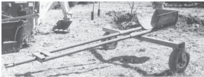
Rig consists of a curved open cradle mounted on two long pipes that pivot on a 2-wheel axle. Trailer is unhooked and then tipped 90 degrees to pick up tree.
