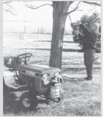
C.F. Marley uses the engine on his garden tractor to belt-drive a generator, which he mounted on front of tractor. It lets him power electric tools such as chain saws and hedge trimmers.
