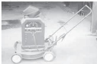
"I came up with the idea of building a frame with casters on each corner. After searching in the shop, I found a lawn mower frame. The engine was bad so I removed it and set the welder on top of the mower's base. I attached two 1 by 4-in. boards to the welder, then bolted it to the mower frame.
