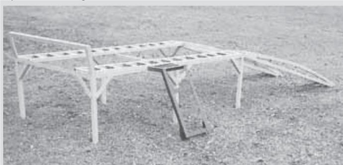
Service rack puts garden tractor up high, making it easy to work on belly-mount mower.
