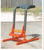
Height of chest pad adjusts from 38 to 60 in. Bottom step adjusts 5 in. in either direction.
