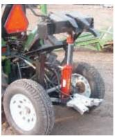
Hydraulic-powered dolly consists of a heavy-duty 2-wheel axle assembly that connects to 3-pt hitch on tractor. Works with 4-wheel drive tractor.
