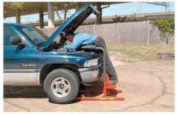
Stool prevents strain to chest, stomach and ribs. When used on side of vehicle, bottom legs strad dle tire.
