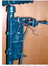
Top handle on trap is raised, left, to cock sharpened spear inside 3/4-in. dia. pipe. Rat trap, right, connects to trigger that runs down to bottom of trap. When mole activates trigger, rat trap instantly releases spring-loaded spear.
