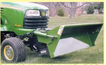
Bucket carries 2 1/2 cu. ft. of material. It fits on front hitch of Deere 425,445, 455 and new X models.
