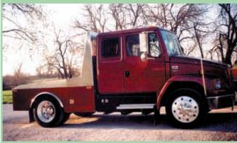
Freightliner cab has bunk behind front seats, a 120-decibel horn on top, and a "western hauler" bed on back fitted with a gooseneck ball.
