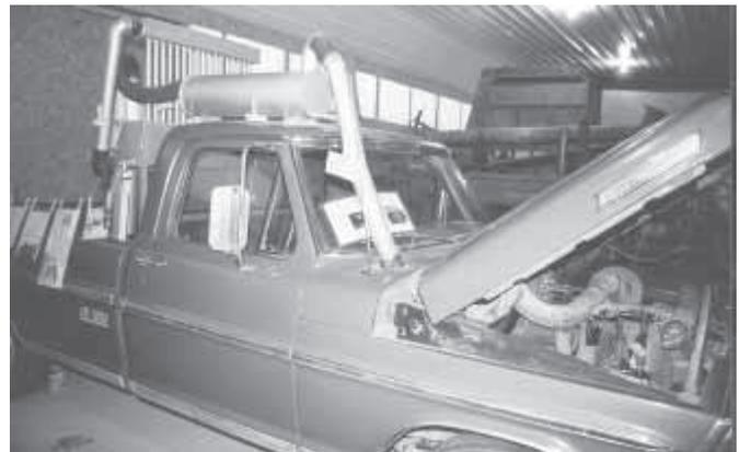
**Housed in Fountain, Minn., this modified 1969 Ford 1/2-ton pickup takes 10 minutes to cook enough wood gas in the combustion chamber to create enough methane gas to run.**
