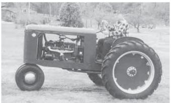
Prototype doesn't have a pto, hydraulics, belt pulley or power lift. It does have a Chevy 216 cu. in. engine, 4-speed transmission, manual shift and two-speed rear end.
