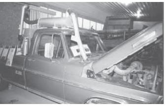
Housed in Fountain, Minn., this modified 1969 Ford 1/2-ton pickup takes 10 minutes to cook enough wood gas in the combustion chamber to create enough methane gas to run.
