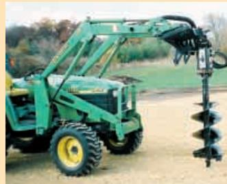
Steel mounting plate accepts skid steer attachments like posthole augers, left. Photo on right shows closeup of mounting plate on loader.
