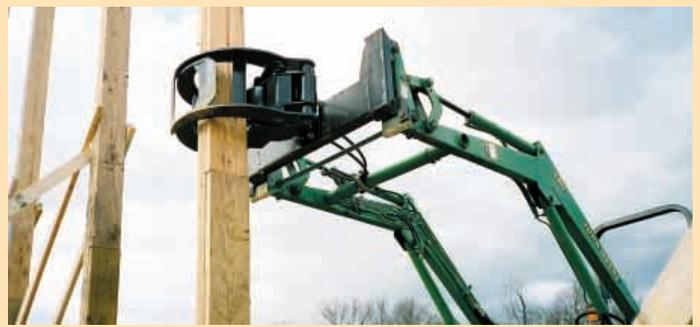
Hitch plate lets you mount any skid steer loader attachment on a tractor 3-pt. hitch or front-end loader, letting you do the work of a skid loader without having to buy one.
