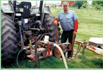
Brent Pitcher built this 3-pt. mounted, pto-driven pressure washer equipped with dual pumps. It has an output of 12 gal. per minute at 3,000 psi.
