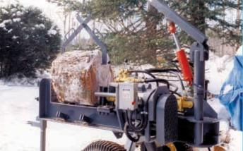
Wood splitter is powered by a 240-volt, 3 hp electric motor that belt-drives a hydraulic pump
