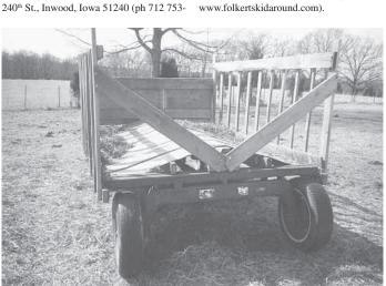
To convert the wagon, the Weinerts built a bulkhead at one end and made wooden feed panels with uprights on 14-in. centers along both sides.
