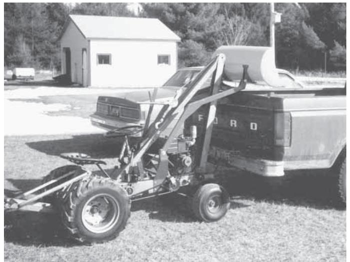
Hartman uses a hand-cranked boat winch to raise and lower loader, and a long trip handle to dump the bucket.
