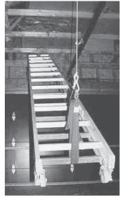
Richard Bergman came up with a pulley and counterweight system that lets him store his 20-ft. extension ladder out of the way above his overhead garage door. Ladder is held up by a counterweight that goes up and down easily.
