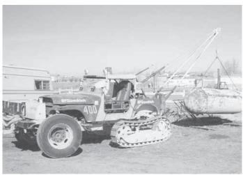
Link Kline's eye-catching "boom truck" looks like a cross between a Jeep truck and a tracked tractor. He uses the rig to lift engines, vehicles or anything else under 8,000 lbs.
