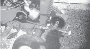
Kenneth Ramey came up with a low-cost sump pump by mounting an old brass pump on his Wheel Horse garden tractor.
