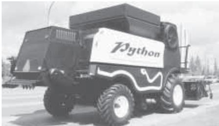
Rite Way's new combine replaced 75 percent of the belts and pulleys found on most combines with hydraulic motors.
